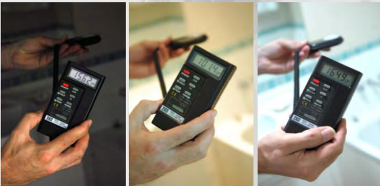
The light meter readings left were taken after just one Solatube Daylighting System was installed into a windowless bathroom
